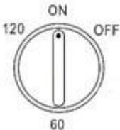
If the timer has set, the fan will automatically stop to the time you have set but within 120minutes the maximum. To operate this timer, please turn the timer switch clockwise to the desired timing position.
