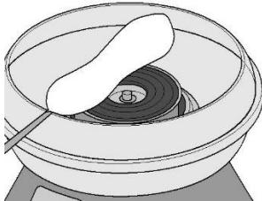
**NOTE:** Do not put the paper roll or wooden stick inside the transparent part, this action can get you burned.
