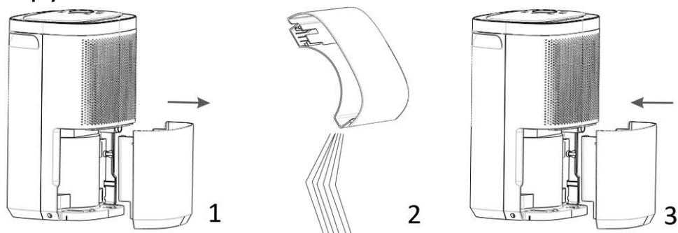
1. Pull out the water tank from the appliance.
