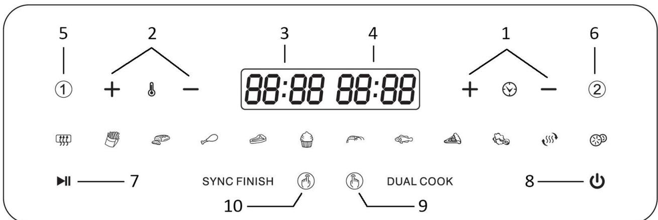
1. Timer control (Press “+” or “-” to adjust the time from 1 to 60 minutes)
